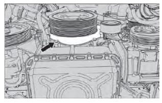
15. Assemble the timing cover front.
