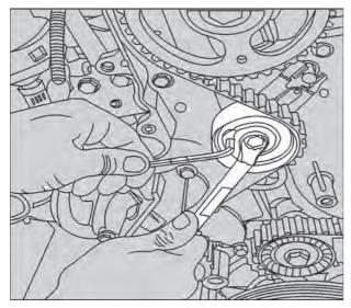
6. Adjust the allen key on the auto tensioner so that the locator remains aligned to the cylindrical pin. (Maximum permissible misalignment + 5°).
