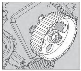
9. Loosen the camshaft gear.
