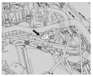
5. Remove the cam phase sensor and insert the locking pin (Part no. 2653 5890 06 09) for on vehicle ease for locking the camshaft
