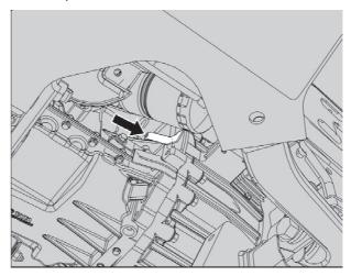
8. Align hole on the HP mounting bracket & lock the gear with the help of locking pin (*Part no. 2653 5890 06 07*).
