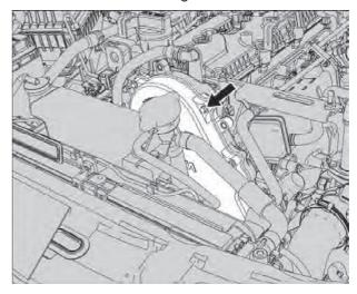
4. Disconnect electrical connection from cam phase sensor and loosen and remove the bolt of cam phase sensor.
