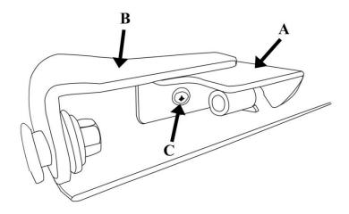
4. Assembly the spring set with tailgate bracket
